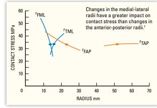
Figure 3b: Optimum Congruency for Minimizing Contact Stress
